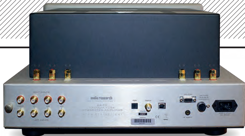
ABOVE: MM/MC phono and three line ins (on RCAs) are joined by optical, coaxial and DSD-ready USB digital inputs. The 4mm speaker connections have 8 and 4ohm taps
